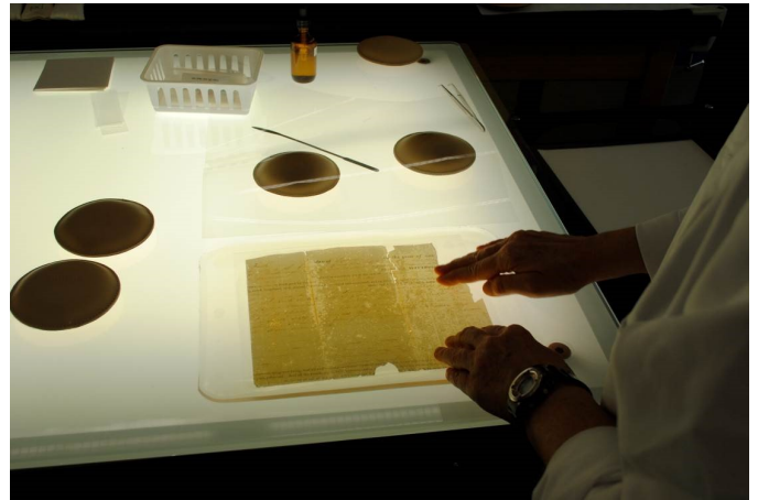
Conservator Silvia Kindl treating indenture with Calcium Phytate in 2% Gellan Gum (Treatment Record, RV360 2012.0006, Image 40)
