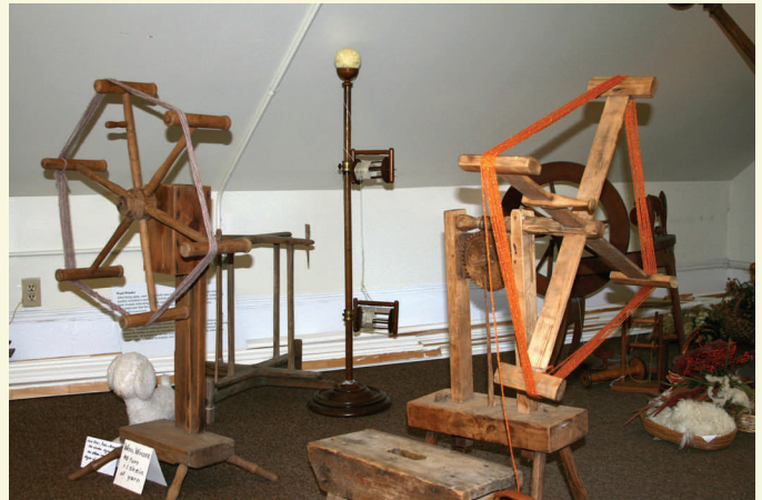
These devices are wool winders. Once the wool is spun it can be wound into skeins to prevent it from tangling and to provide a measure of length. A skein is defined as "a length of thread or yarn wound in a loose long coil". For the two wool winders above forty turns provides the length that was described as a skein. Each of these winders has a mechanical mechanism that indicates forty turns so the operator doesn't have to count.
